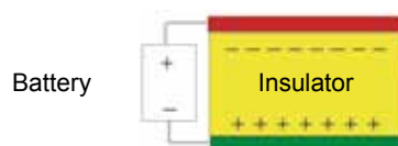
Picture 5: Charge separation through influence
